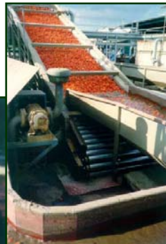
INOXALL SWP final washing and elevating
