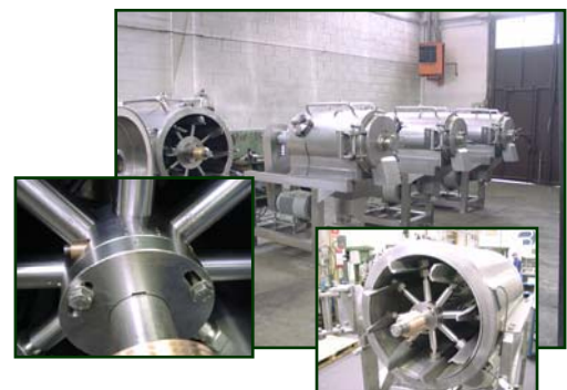
High-speed refiner TURBOMAX , famous for its flexibility and capacity up to 30 tons per hour.
