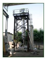
Depending on the final °Brix to be reached, puree can either be concentrated by our plate evaporator FRUMACO (right) or our LUBER (left). The Luber is designed to concentrate in a single fast passage either thermo-sensitive liquidor highly viscous products.
