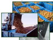
From the washing tank the fruits enter the sorting line **SELINOX** (left), consisting of a roller belt conveyor which allows to inspect the fruits very carefully.
