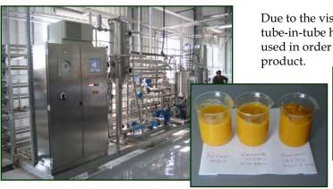
Due to the viscosity of fruit puree, tube-in-tube heat exchangers are used in order to sterilize the product.
