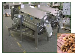
Stone cleaner JUMBOCREAMER Single stage pulper of big capacity and particular sturdiness fitted with interchangeable screens for pulping, refining or pitting operations of ripe, chopped or pre-cooked fruits. Complete with inverter.
