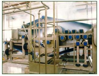
**BELT PRESS:** It is possible to recover up to 75% of juice with a single pressing or more than 85% with a double pressing.
