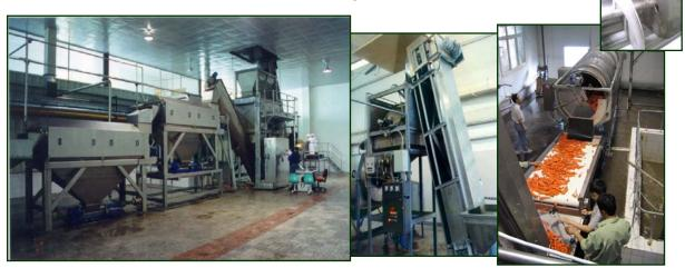
In a two-step sequence of loosening the carrot's skin by steam and brushing it off together with water, the carrots are prepared for their conversion into the final product. Bertuzzi has always worked very successfully with this technology and it is especially recommended when the final product is addressed to the baby-foods preparation.
